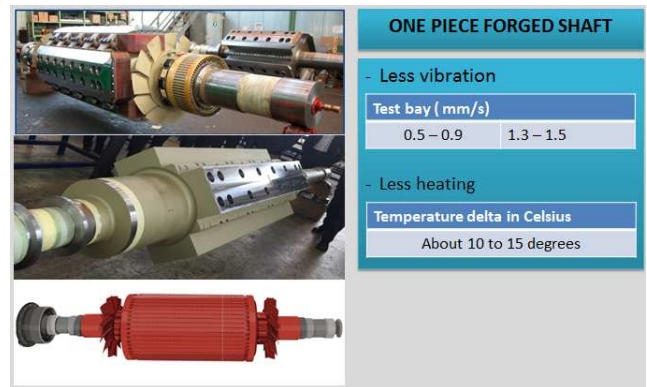
Figure 6. Rotor Construction.
